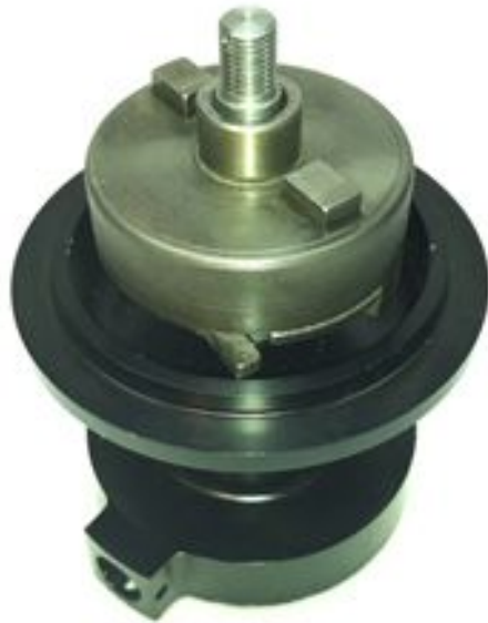
Figure 4: Impulse Coupler and Faux Impulse Coupler Installed. Step 4c
