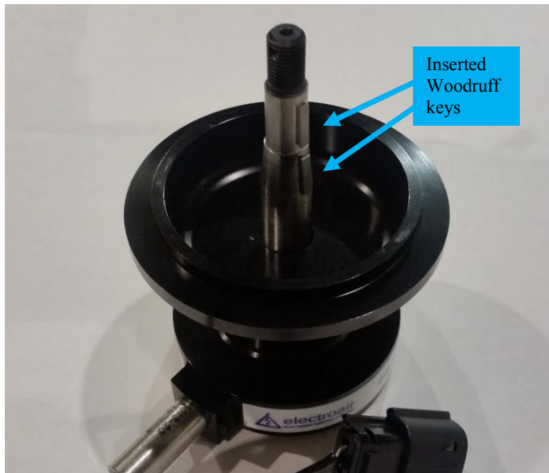
Figure 3: Impulse Coupled MTH Shaft with Woodruff Keys Inserted. Step 4b
