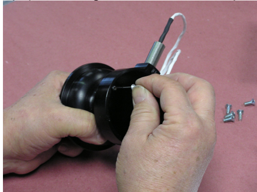
Figure 28: Installation of MTH Alignment Pin
