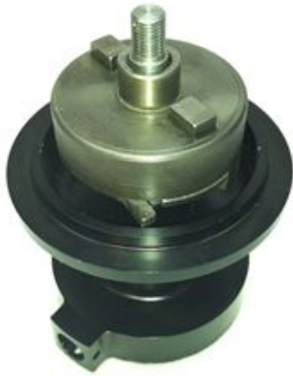
Figure 25: Impulse Coupler and Faux Impulse Coupler Installed. Step 4c
