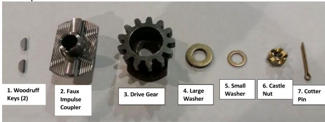
Figure 6: Install Order of Components to Impulse Coupled Shaft.
